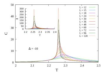
FIG. 4. Specific-heat (main panel) and magnetic susceptibility (inset) curves corresponding to Eqs. (4) and (5) at  $\Delta = -10$  from Wang-Landau simulations. After an increase in the system size, the location of the peaks shifts to the left.
